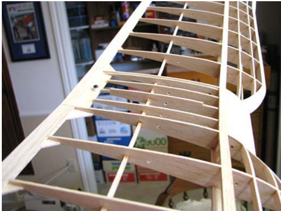
This picture shows the center section planking completed.
